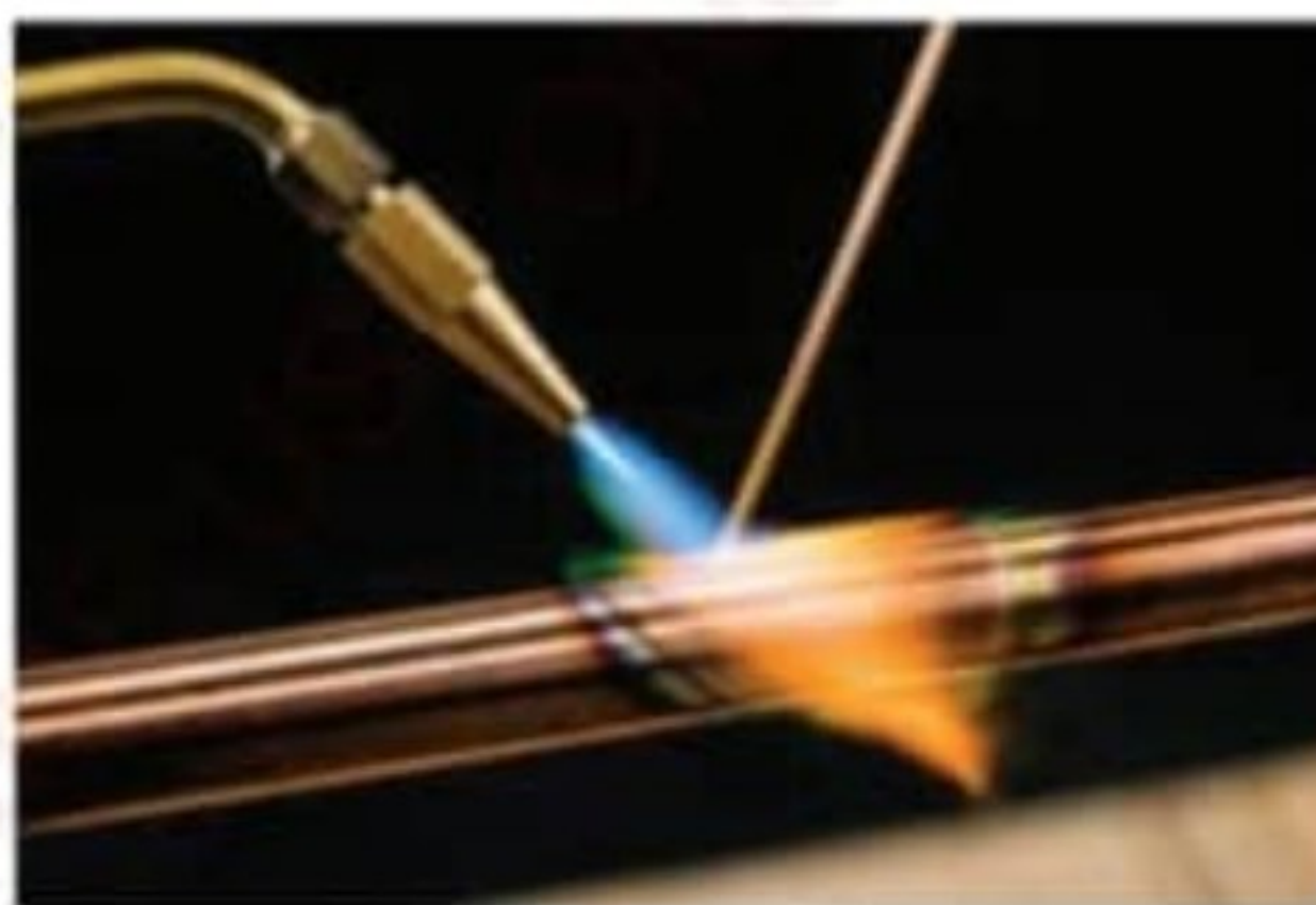
Figure 2.9: Welding of metals using oxy-hydrogen flame
