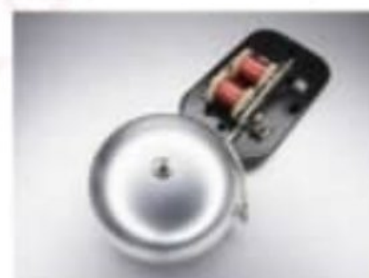
(b) Photo of an electric bell
